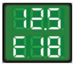
Fault codes are used to indicate that a fault has occurred in the equipment. They are given in the lower part of the display with an E followed by a fault code number.
