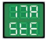
When mains power is supplied, the unit runs a self diagnosis of the LEDs and the display. The program version and panel version, "Steel", "Alu", "Steel NA" or "Alu NA", are presented. (In this example the program version is 0.17A and the panel version is "Steel".) (Long texts are automatically scrolled in the display.)
